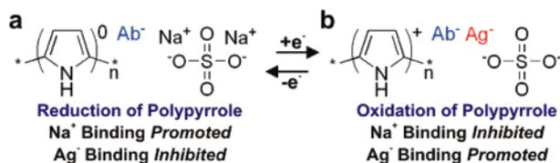
**Figure 1.** Oxidation and reduction of PPy doped with negatively charged antibodies (Ab<sup>-</sup>) and sulfate polyions (SO<sub>4</sub><sup>2-</sup>) in a physiological salt buffer. During reduction of PPy (a) negative charges in the polymer are neutralized via interactions with Na<sup>+</sup> ions. Conversely, during oxidation of PPy (b) binding of negatively charged antigens (Ag<sup>-</sup>) is facilitated such that the polymer remains in a charge neutral state.
