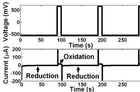
**Figure 4.** Typical current response of  $\alpha$ FN-doped PPy during repeated oxidation and reduction in a NT solution.
