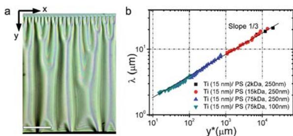
**Fig. 4** (a) Optical micrograph of a wrinkled domain obtained after immersion in toluene vapors of a Ti/PS/SiO<sub>x</sub> multilayer formed by a 15 nm thick titanium layer deposited on a 0.25 μm thick polystyrene layer ( $M_w = 15$  kDa) on top of a silicon substrate. (b) Evolution of the wavelength *versus* the distance from the diffusion front for different low molecular weight polymers.
