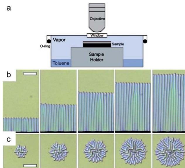
**Fig. 1** (a) A schematic representation of the experimental set-up. From left to right: Successive optical micrographs of (b) the growth of parallel and (c) radial wrinkled domains, obtained after immersion of a Ti/PS/SiO<sub>x</sub> trilayer in toluene vapors. The scale bar corresponds to 20 μm.
