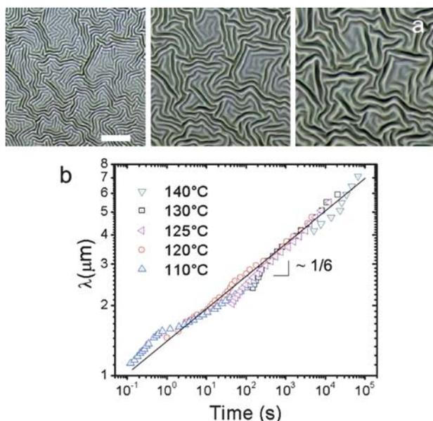
**Fig. 5** (a) Thermal wrinkling. Optical micrographs of the temporal evolution of wrinkled Ti(15 nm)/PS(250 nm; 15 kDa)/SiO<sub>x</sub> trilayers after 1, 2 and 30 min at 130 °C, from left to right, respectively. The scale bar corresponds to 20 μm. (b) Evolution of the wavelength *versus* time of wrinkled Ti(15 nm)/PS(250 nm; 15 kDa)/SiO<sub>x</sub> at different temperatures. Curves were shifted thanks to the time–temperature principle (Williams-Landel-Ferry (WLF) equation).
