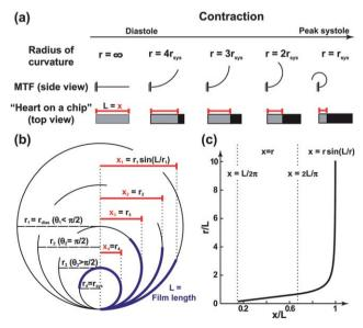
**Fig. 2** Calculation of the radius of curvature. (a) A schematic drawing contrasting the view of the regular MTF assay with the "heart on a chip", through the contraction cycle; (b) The *x*-projection measured during the running of the assay, as the radius of curvature increases; (c) Plot showing the relationship between the measured *x*-projection and the radius of curvature, with appropriate equations to use in each region.
