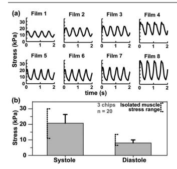
**Fig. 3** Cardiac contractility recorded with "heart on a chip". (a) Stress traces for each film from chip in Fig. 1d; (b) stress summary for 20 films in 3 chips compared to isolated right ventricular muscle(dashed lines);<sup>33</sup> PDMS layer thicknesses for three chips: 18.6, 15.6, 14.5 μm.
