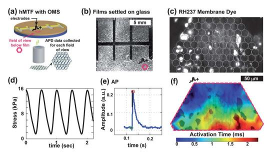
Fig. 5 Contractility and electrophysiology experiments: (a) Chip in OMS. (b) Brightfield image of a chip marked with a field of view (fov) (PDMS layer = 23μm); (c) RH237 membrane dye image, overlaid with the fiber array location (outlined as fov in (b)). (d) Example stress trace from two chips. (e) Mean optical AP trace. (f) Activation map plot (blue to red contour plot) over an image of the RH237 dye (in black).
